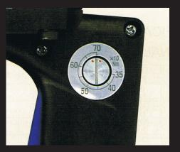
**5.** Squeeze trigger switch. When required torque has been reached, wrench stops and tightening is over.
