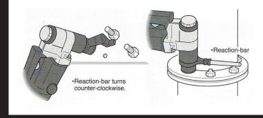
Press trigger intermittently until the reaction-bar touches the prop (support)
